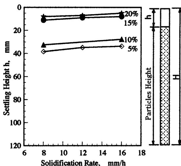
Figure 4 Relation of settling height with solidification rate and particles content.
