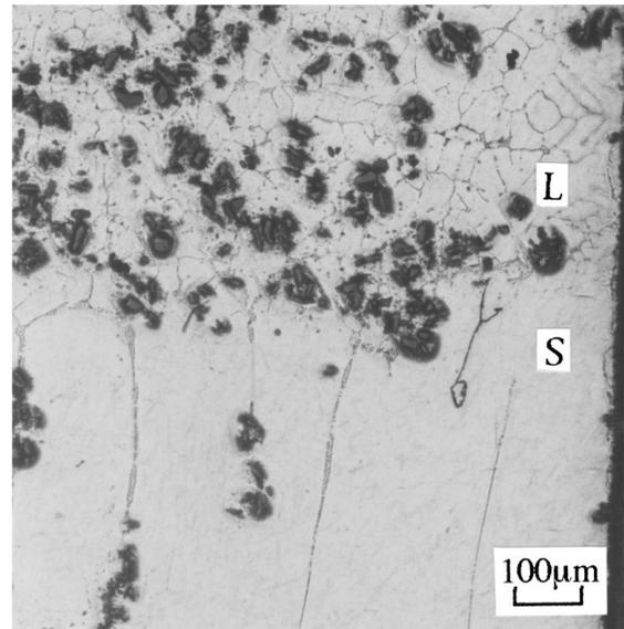
Figure 6 Particle distributions at S/L interface for  $\text{Al}_2\text{O}_3/\text{Al}$ -Ce composites. (Upward freezing.  $V_f = 5$  vol.%,  $R = 2$  mm/h).
