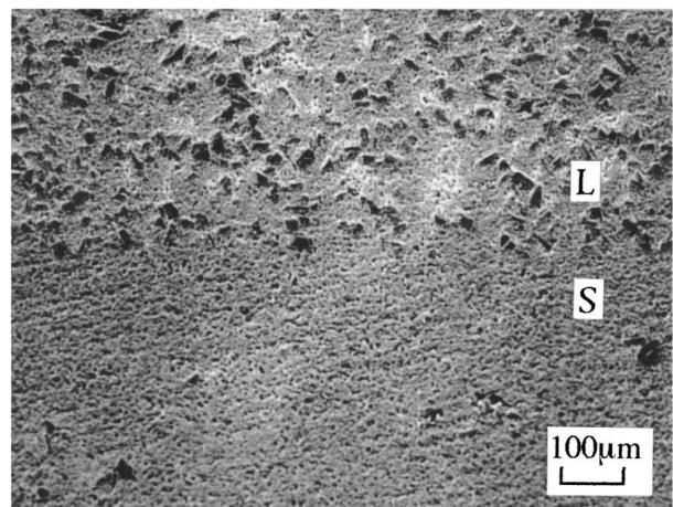
Figure 7 Particle distributions at S/L interface for a more purified  $\text{Al}_2\text{O}_3/\text{Al}$  composites. (SEM; upward freezing.  $V_f = 7$  vol.%,  $R = 2$  mm/h).
