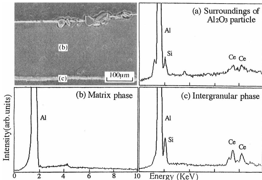
Figure 8 SEM and EDX analysis for  $\text{Al}_2\text{O}_3/\text{Al-Ce}$  composites.
