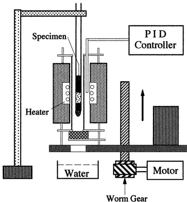
Figure 1 Schematic representation of the zone UDS apparatus.
