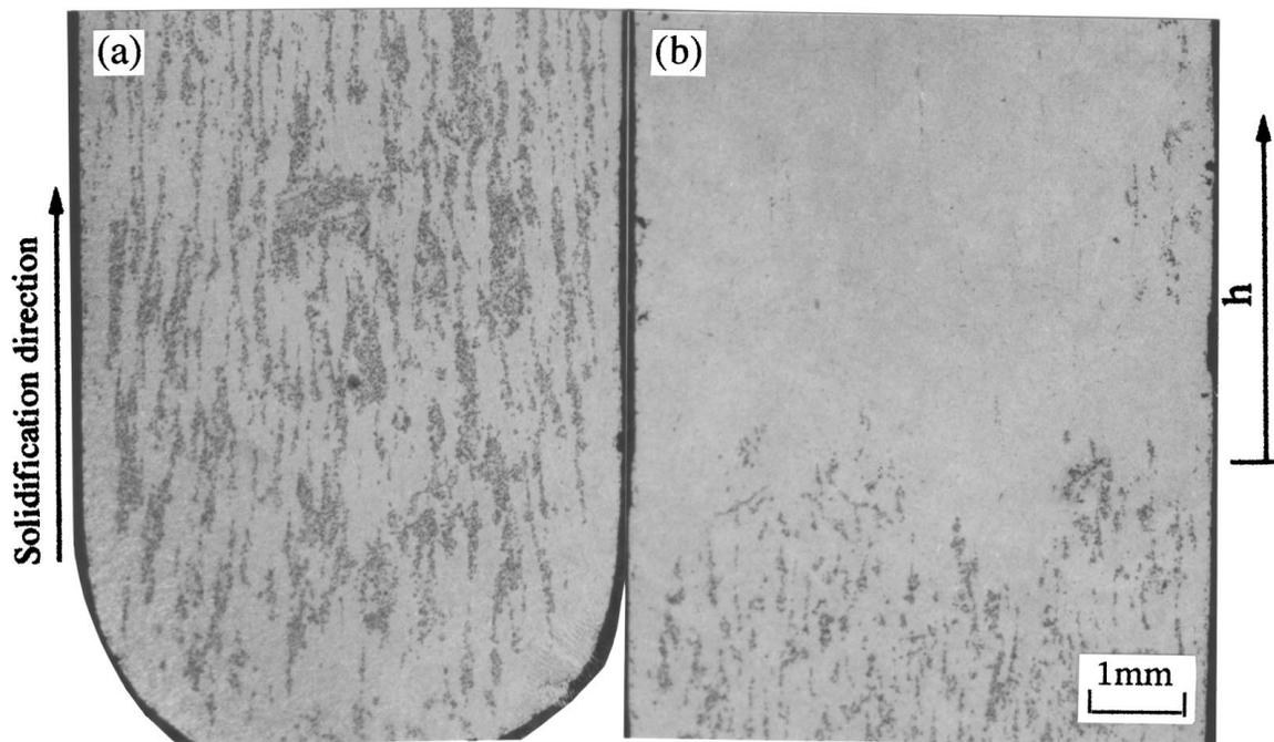
Figure 3 Representative macro-distribution of particles after freezing of the whole sample. ( $V_f = 10$  vol.%,  $R = 16$  mm/h). (a) Lower part; (b) Upper part.
