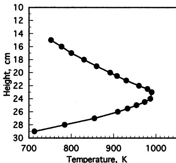
Figure 2 Temperature profile of the zone melting furnace.
