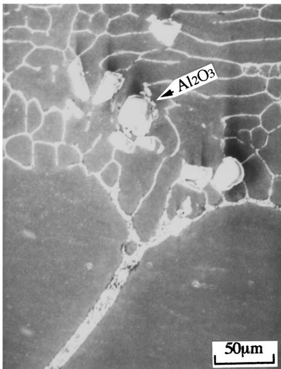
Figure 5 Interfacial morphology and Particle distributions for  $\text{Al}_2\text{O}_3/\text{Al}$ -Ce composites. (SEM; upward freezing.  $V_f = 2$  vol.%,  $R = 2$  mm/h).
